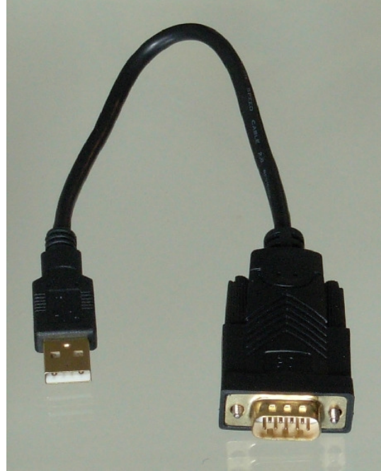
Current type with FTDI chipset
