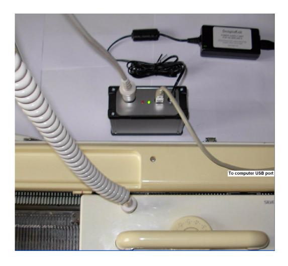
This cable link enables DesignaKnit to control interactive knitting on the Silver Reed modular electronic knitting machines SK830, SK840, SK860, & SK890, and also on the Knitmaster 550, 560, and 580 machines.
